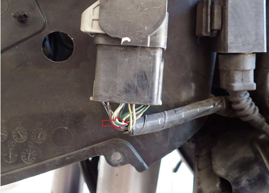
Picture of 23PIN OEM connector shown. The yellow/green wire which needs to be soldered to the second wire from the right (red arrow).
